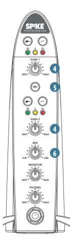
USB: The signal from Tracktion arrives via USB, and is sent directly to your monitors, headphones, and SPDIF output. If the MIX knob is set to USB, you will only hear the output from Tracktion (or other audio software).
